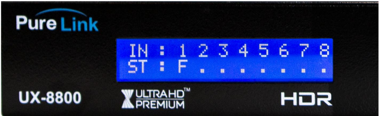
< PIC. External EDID – Signal Status >
